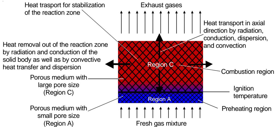
**Fig. 2: Heat transport mechanism**
