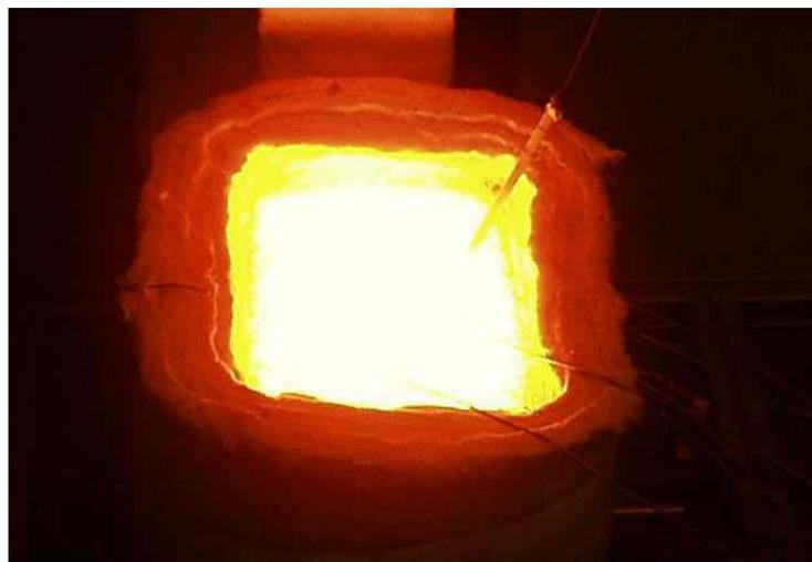
**Fig. 3: Gas infrared porous burner RADIMAX in operation**
